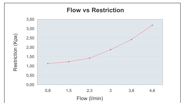
FH 232 Series with FS 19785 (25 µm) Filter element per SAE J905
